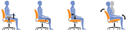
Arm Height Adjustment Waterfall Seat Edge Properly Contoured Cushions Center Tilt Movement
